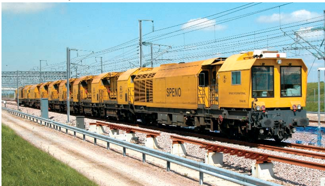
BELOW: One item of track machinery not often seen is the new Speno rail grinder No RR48M2. The unit is pictured at Singlewell Loops on Phase One of the Channel Tunnel Rail Link on 15th May 2005. Work is now well underway on CTRL Phase Two which will link the existing section with Stratford International and London St. Pancras. The company building Phase Two, London & Continental Railways (LCR) has admitted that the project is now overbudget after construction costs spiralled. PATRICK SEALE
