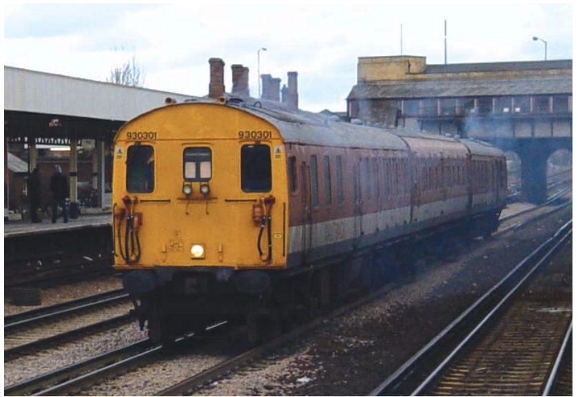
ABOVE: The recent cold snap has seen Network Rail's 'De-icing' units out and in action on the Southern Region. Here 3-Car No. 930301 passes Tonbridge on 20th February, making a rare daylight appearance. COLIN PRICE
