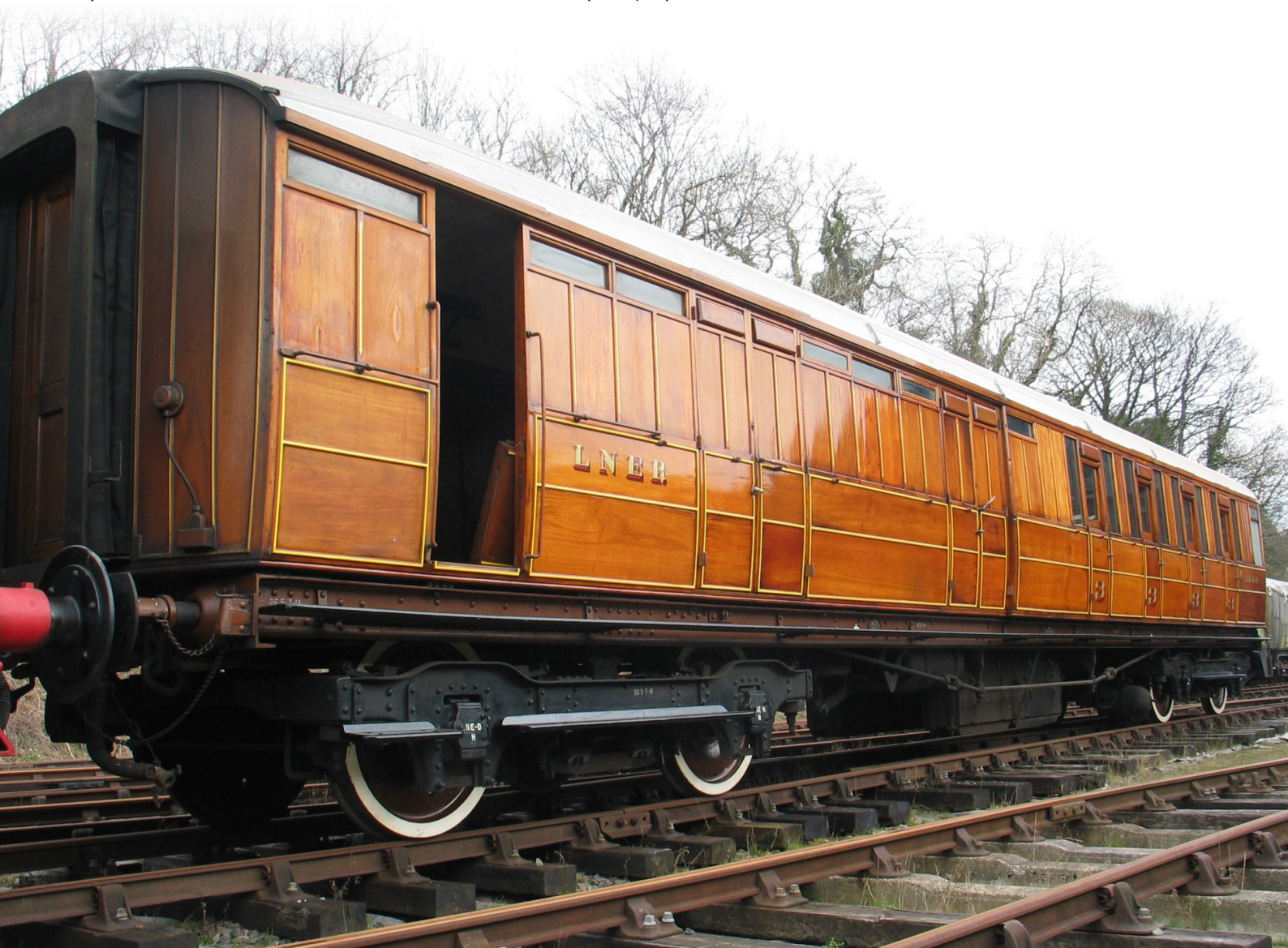
Below: Gresley Corridor Brake Third No. 3669, which was built by the Birmingham Railway Carriage & Wagon Company in 1930, is privately owned by members of the LNER Coach Association and recently arrived at Kirkby Stephen East. It has been receiving attention to the roof, wheelsets and stepboards and is currently undergoing lining out and varnishing. The non-corridor side is visible in this view. Stainmore Railway Company
