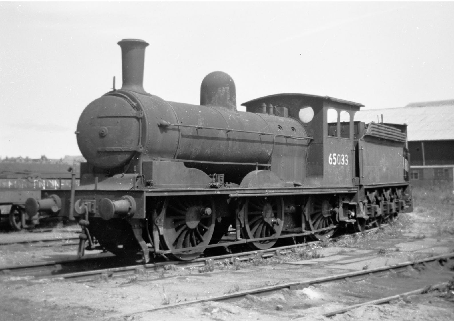
Below: No. 65033 looked much more forlorn at Darlington by the time it was finally towed away to Consett steelworks. Gone are the smokebox dart, vacuum hose and coupling rods, the latter having been removed to ease shunting. LCLT Collection
